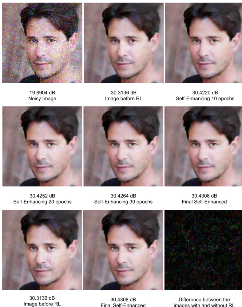
Figure A5: Recursive Self-enhancing RL Visualization: the figure shows how the test images are recursively enhanced in a 50-epoch RL training. We observe a performance boost when iterating the weights of decomposed transformations under three latent subspaces. With the reinforcement learning agent, the network converges to a better result compared to the case where only a solo VAE framework can achieve. The last line also specify the difference between the starting image we fed into RL agent and the final result after recursive learning.
